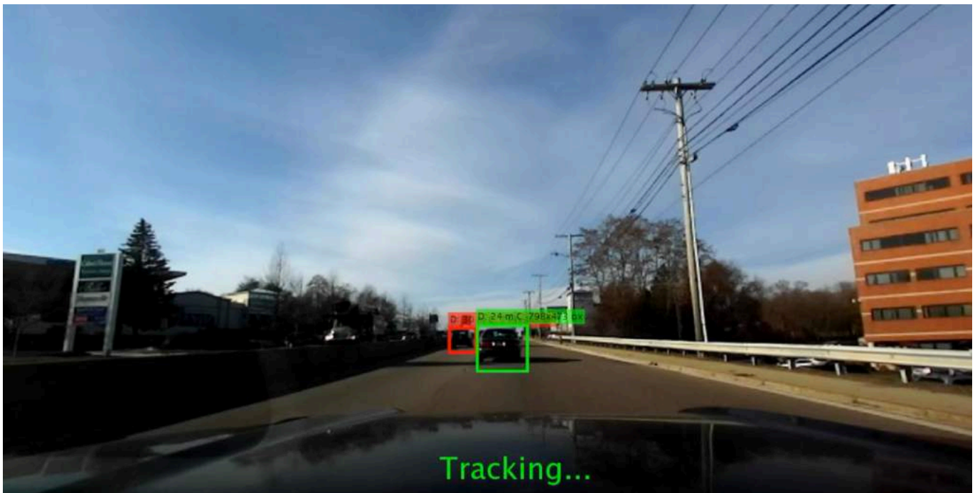
FIGURE 2 VEHICLE SUCCESSFULLY DETECTED (GREEN) AND ANOTHER (RED) WHICH IS NOT OF INTEREST
