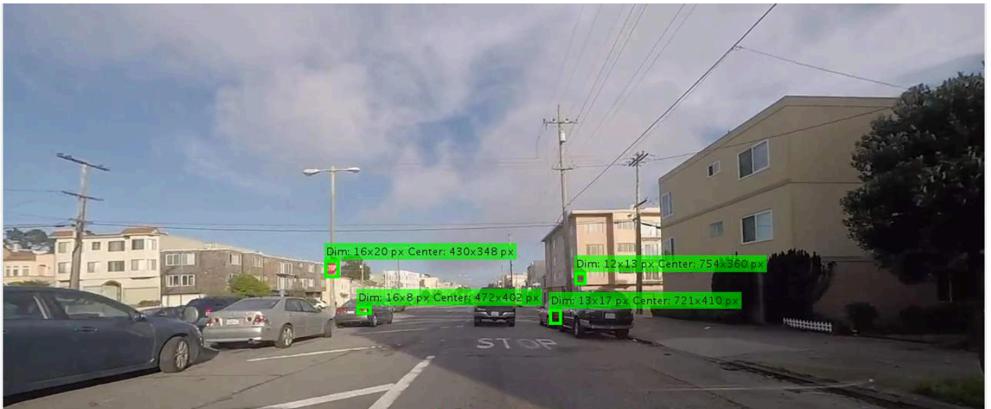
FIGURE 8 SHOWS FALSE POSITIVES OF COLOR DETECTOR
