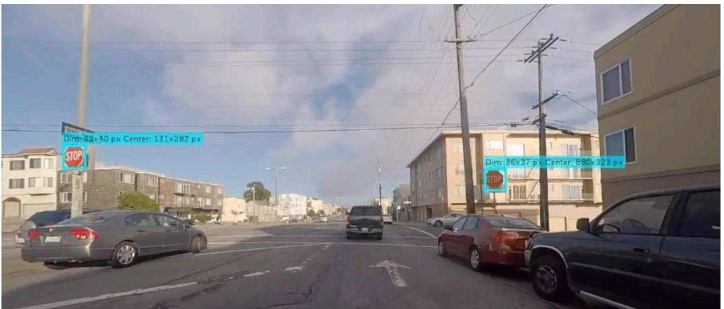
FIGURE 9 STOP SIGN DETECTION USING ONLY THE CASCADE DETECTOR
