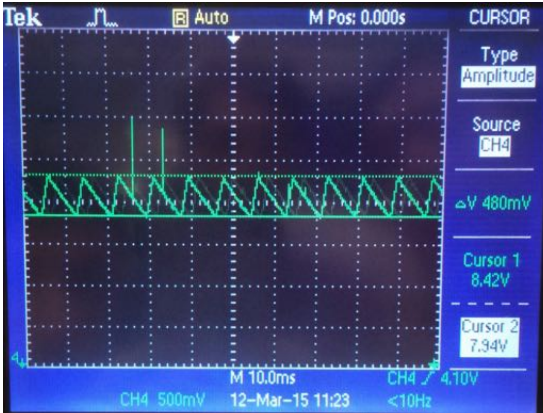
Figure - 3. Rectifier ripple voltage approximately 480 mV
