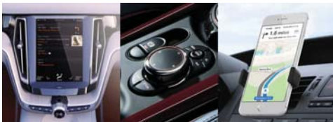
Figure 2: Built-in vehicle touch screen (Left), capacitive based console controller (Middle), smartphone (Right)
