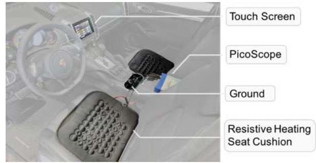
Figure 3: Carpacio data collection setup
