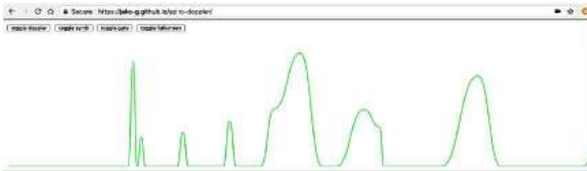
Fig. 10.2: A screenshot of the open source ultrasonic Doppler based motion magnitude visualizer
