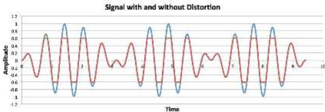
Fig. 6.3: An example showing the distortion due to clipping sinewave
